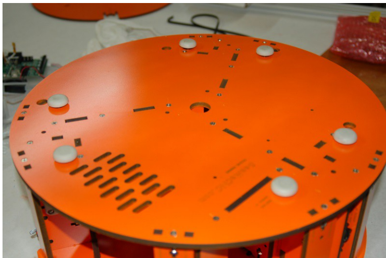
Fig. 2-40: Screws tightened and shoes installed.
