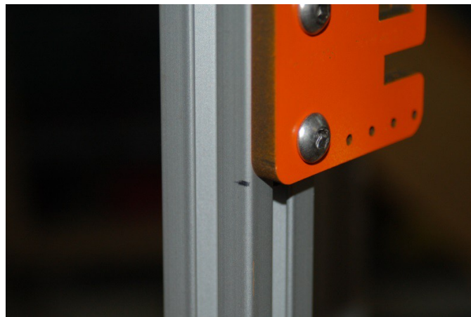
Fig. 4-2: Marking the bottom of the Idler Mount.
