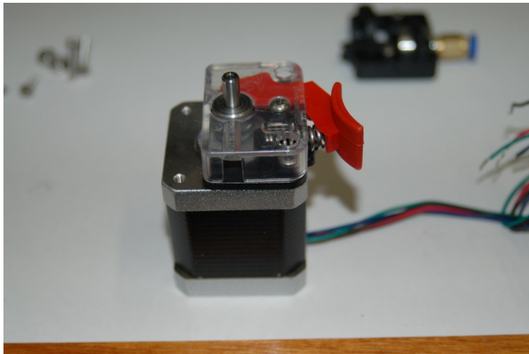
Fig. 12-8: Filament release installed.
