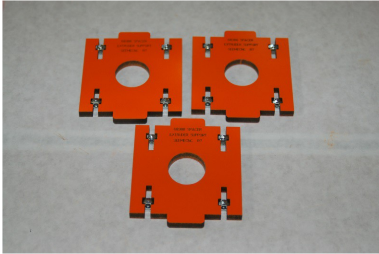
Fig. 11-3: Nuts installed in the extruder supports.
