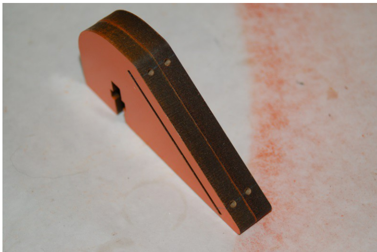
Fig. 16C-3: Pilot holes for mounting the LCD panel.
