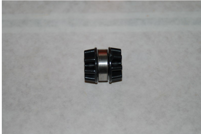
Fig. 2-20: Idler bearing assembly ready to install.
