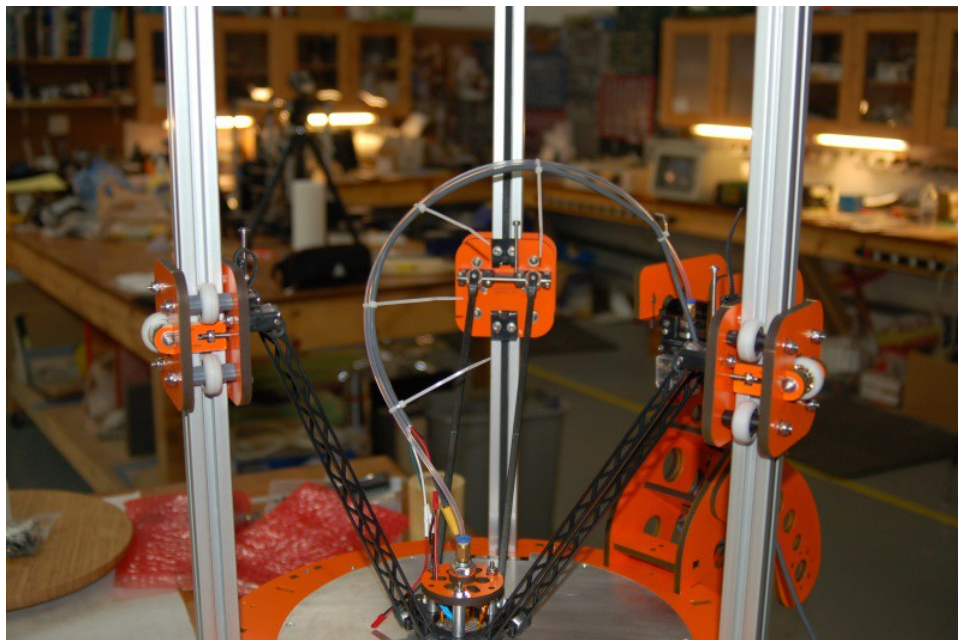
Fig. 16-9: Hot end wiring attached.
