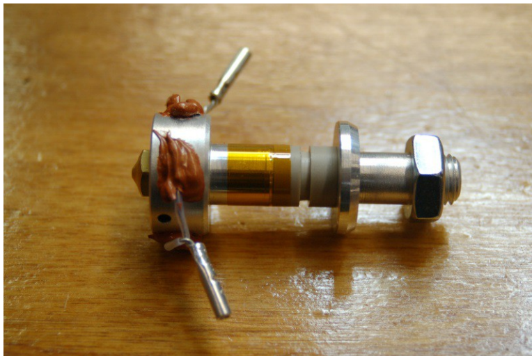
Fig. 15-6: Kapton wrap on the PEEK barrel.
