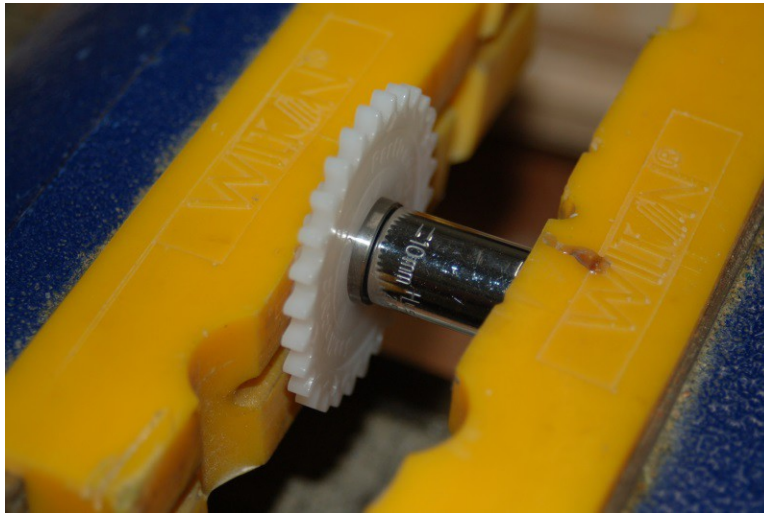
Fig. 12-1: Installing the bearing in a Steve's Extruder gear.
