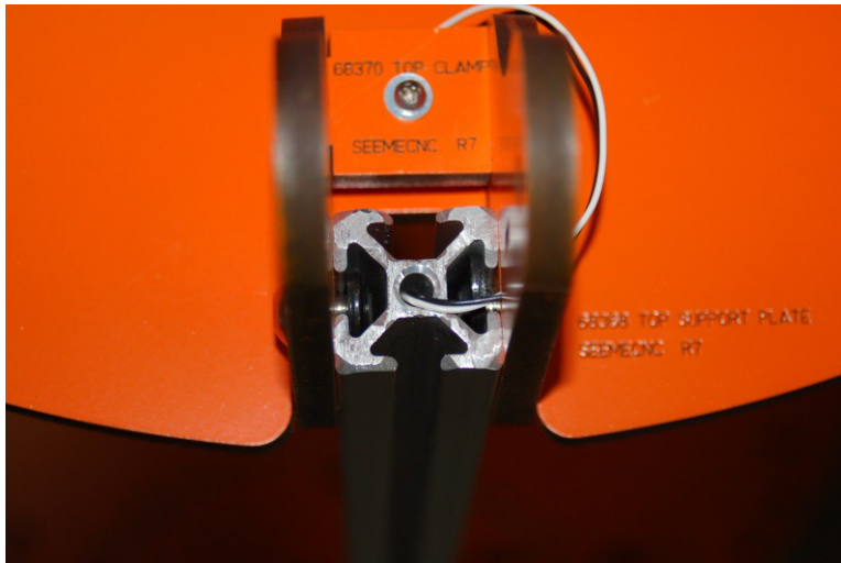
Fig. 6-4: End stop wires routed through the tower extrusion. (Step #3)
