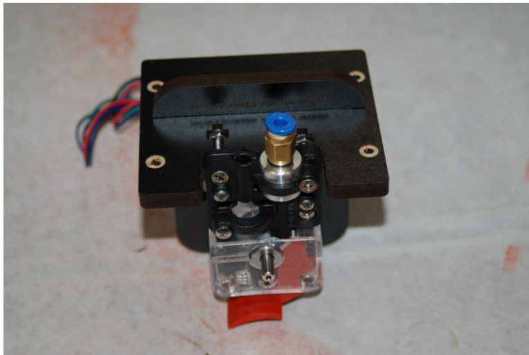
Fig. 12-13: EZStruder mounted to the adapter plate.
