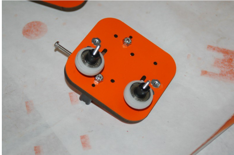
Fig. 7-13: Finally, add two more conic shaped spacers as shown.
