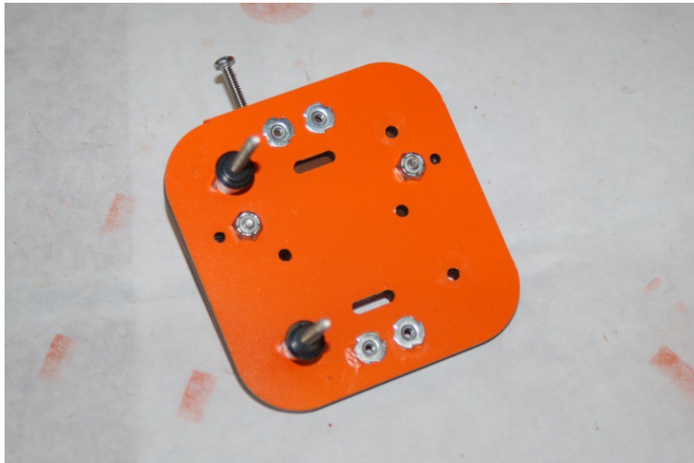
Fig. 7-11: The spacer stack begins with a black, conical spacer.
