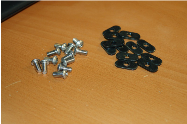
Fig. 3-1: Screws and T-Slot nuts required for the tower installation.
