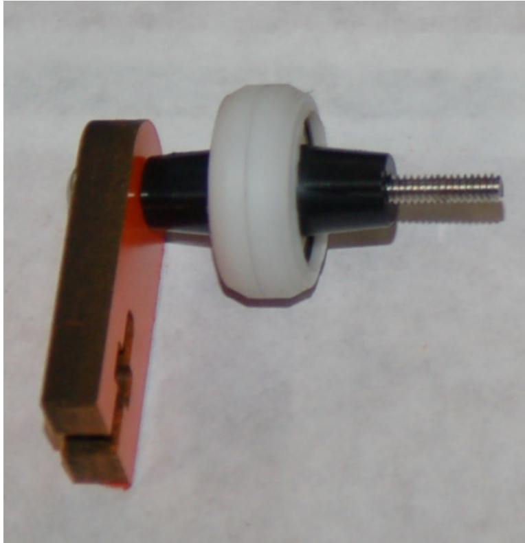
Fig. 7-22: Install two conical spacers and a bearing assembly.
