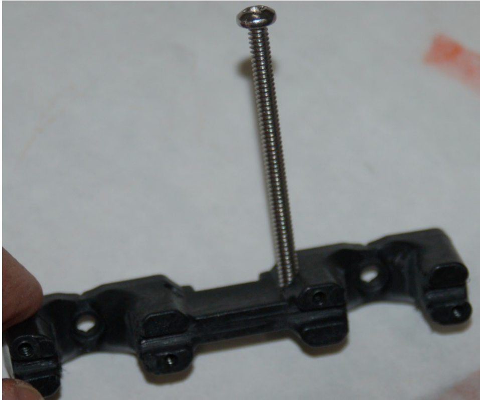
Fig. 7-6: End stop adjustment screw installed in the u-joint mount.
