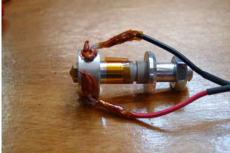
Fig. 15-7: Attaching the power leads to the hot end.
