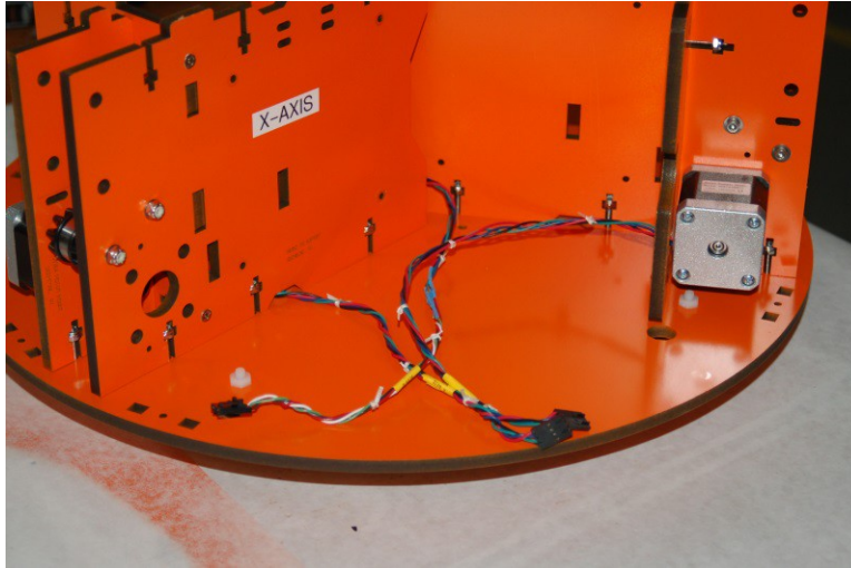
Fig. 2-30: Stepper motor wire routing.
