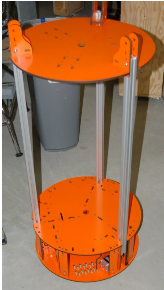
Fig. 5-5: Assembly progress so far.
