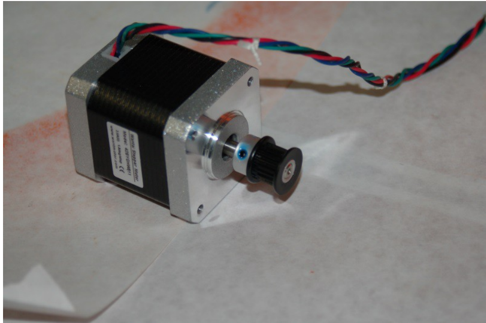
Fig. 2-10: Drive gear installed.
