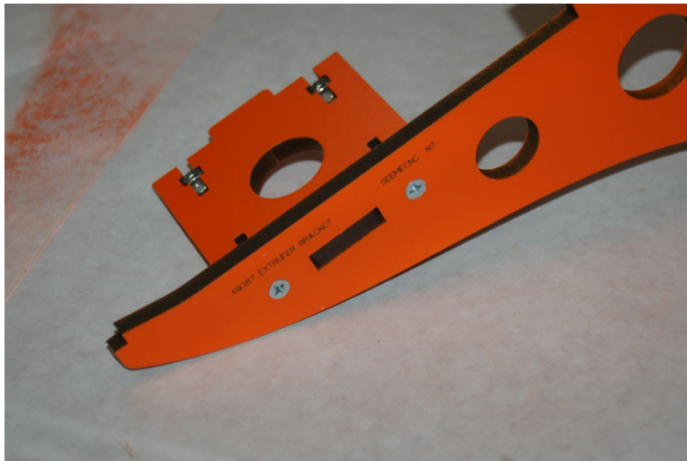
Fig. 11-4: Installing the first extruder support.
