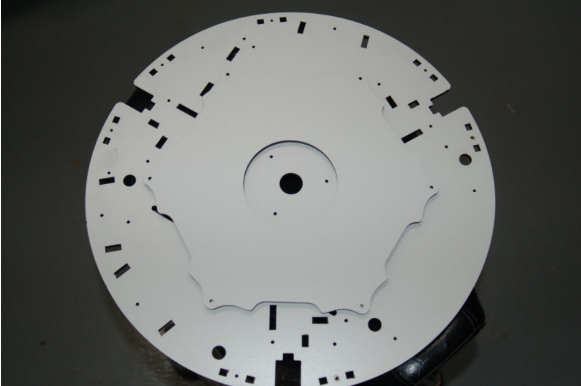
Fig. 2-36: Using the heated bed spacer plate as a hole locator.
