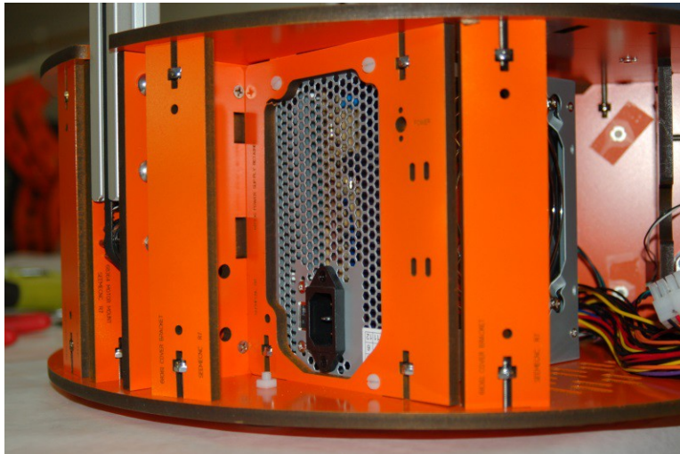
Fig. 13-3: Power supply mounted.
