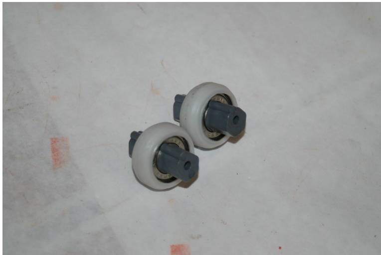
Fig. 7-17: Bearing assemblies with eccentric cams in place
