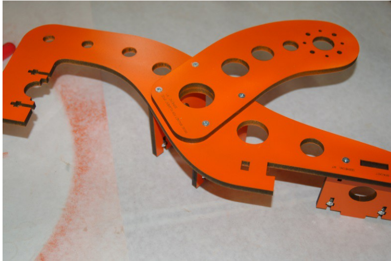
Fig. 11-5: Spool holder installed on extruder bracket.
