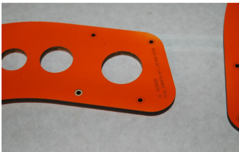
Fig. 11-2: Extruder bracket with one of the countersinks popped out.
