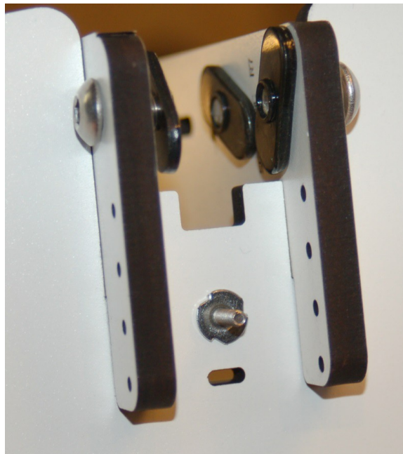
Fig. 4-8: Bottom view of the Idler Mount installed in the Top Support Plate.
