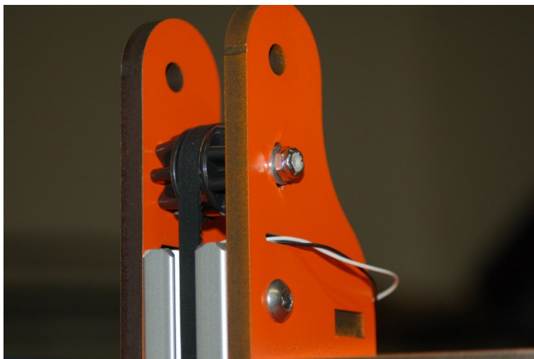
Fig. 8-11: Screw at center point of adjustment travel.
