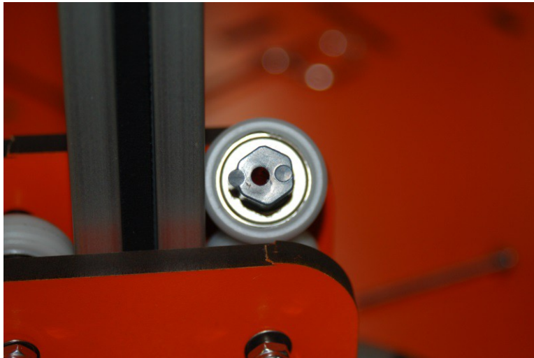
Fig. 7-18: Correct orientation of the eccentric cam prior to installation.
