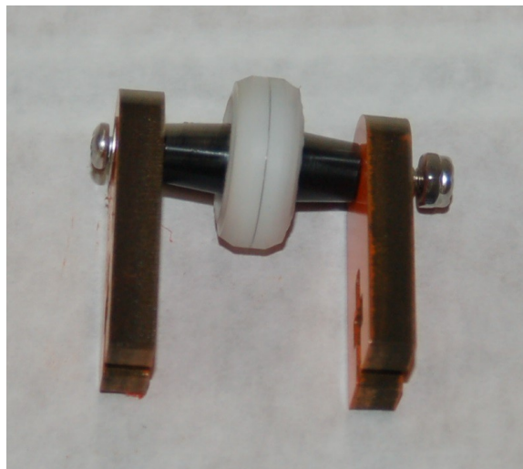
Fig. 7-23: Next, install the remaining Axle Support, a washer and a #6-32 nylon lock nut.
