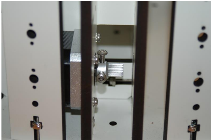
Figure 22 - Pulley correctly installed
