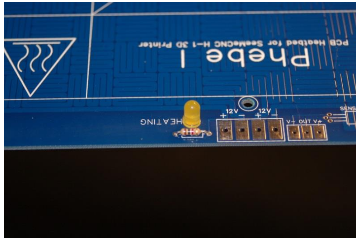
Figure 94 - Power LED installed.
