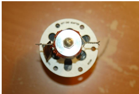
Figure 106 - Resistor wires wrapped together.
