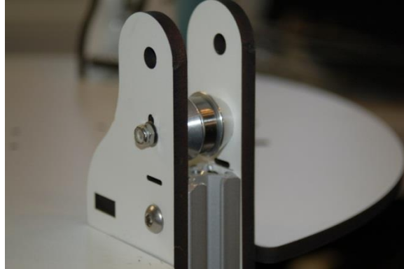
Figure 78 - Upper Idler Bearing Installed
