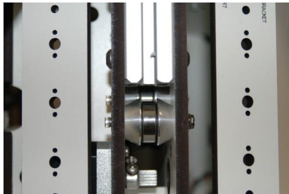
Figure 77 - Lower Idler Bearings Installed
