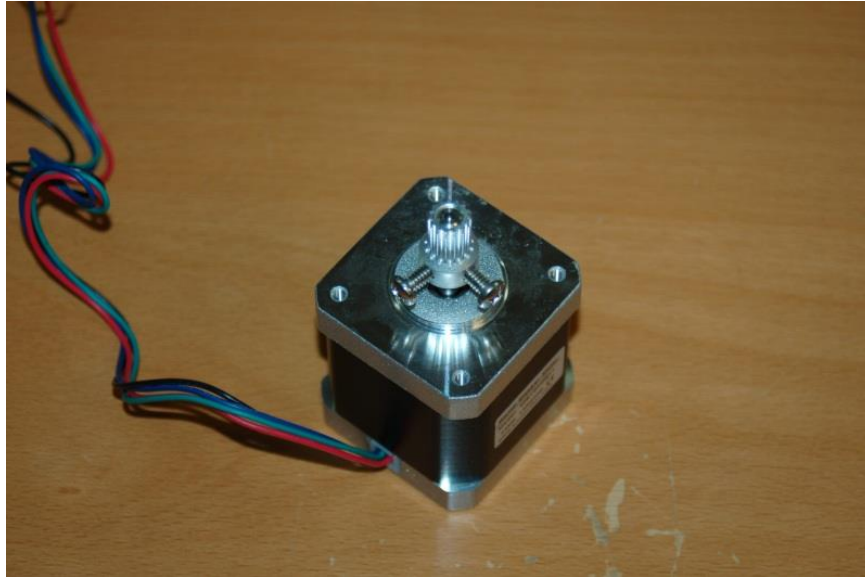
Figure 19 - Belt Pulley Installed
