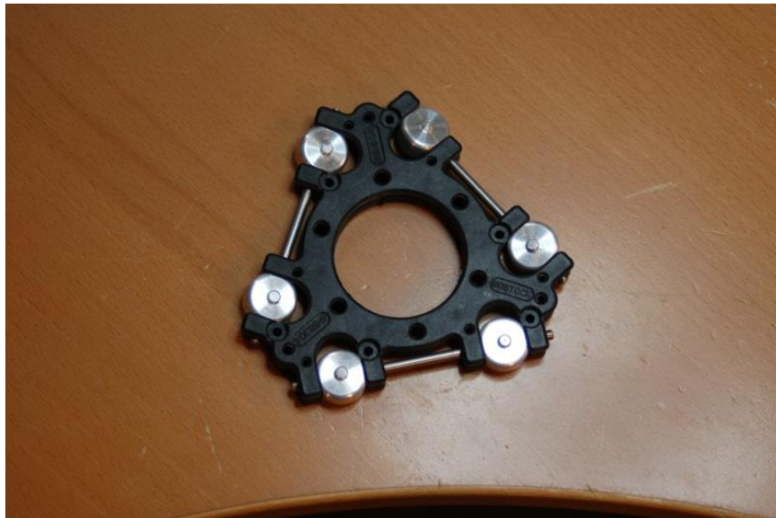
Figure 48 - U-Joints and U-Joint Axles Installed.
