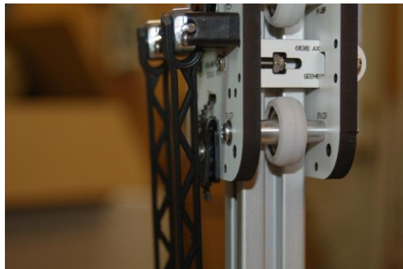
Figure 81 - Belt Clamp Installed
