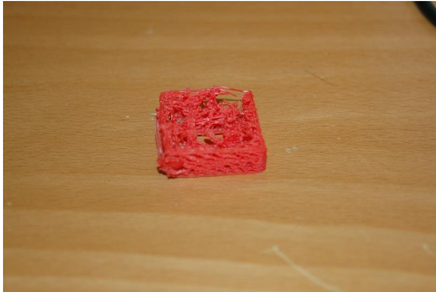
Figure 155 - Too fast, not enough plastic.
