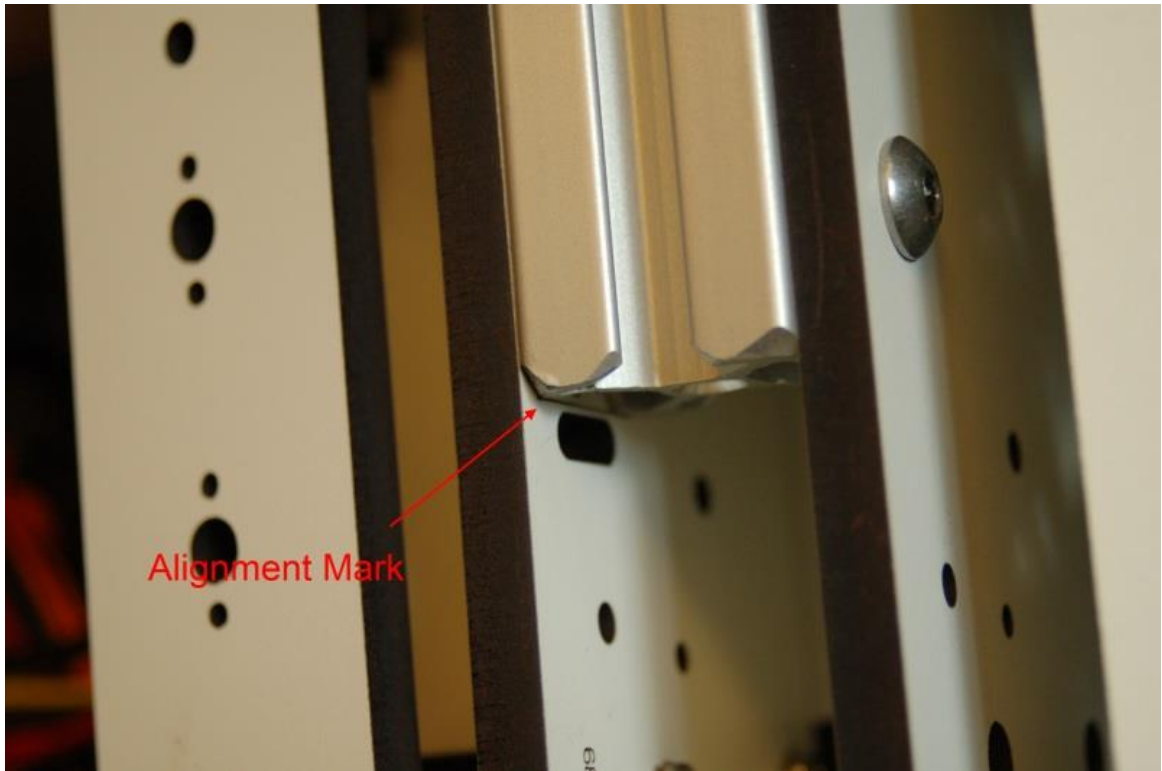
Figure 37 - Rail Bottom Aligned with Mark
