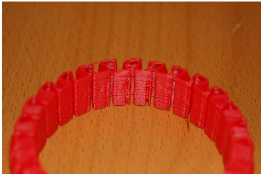
Figure 157 - Stretchlet, too fast.
