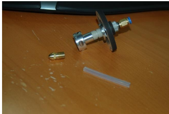
Figure 102 – The Teflon Liner ready for installation.
