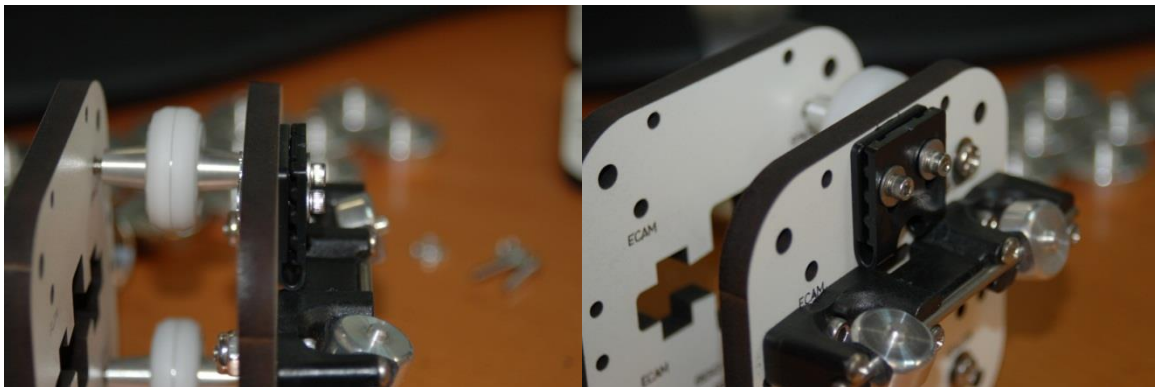
Figure 67A & Figure 67B – Upper Belt Clamp Installed
