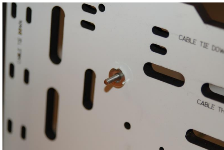
Figure 25 - Installing the T-nuts, back side
