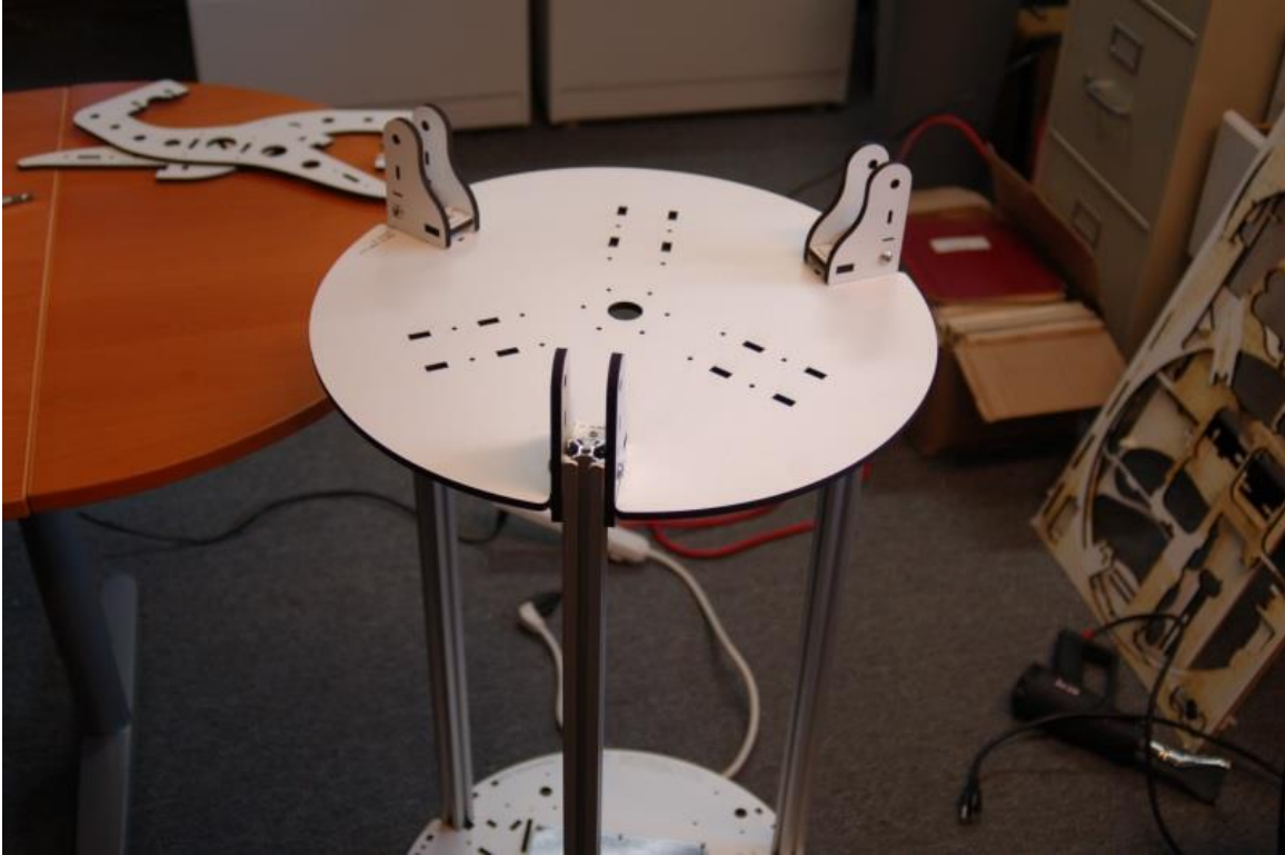
Figure 36 - Top Support Plate Installed
