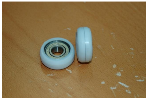
Figure 59 - Bearings with Acetal Sleeve Installed.
