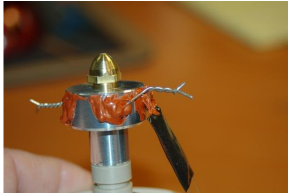
Figure 105 - Resistor wires wrapped together.
